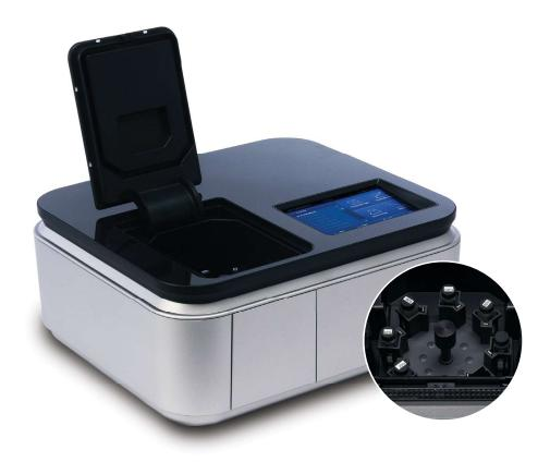
OPTIZEN POP offers four measurement modes (Photometric Mode, Quantitative Mode, Spectrum Mode, Kinetics Mode). The user can choose a suitable mode depending on the purpose to measure. The embedded S/W, touch screen interface and application facilitate the use of the device.
