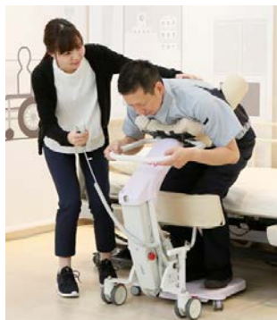
Mobility Support Robot to support transferring and standing position
