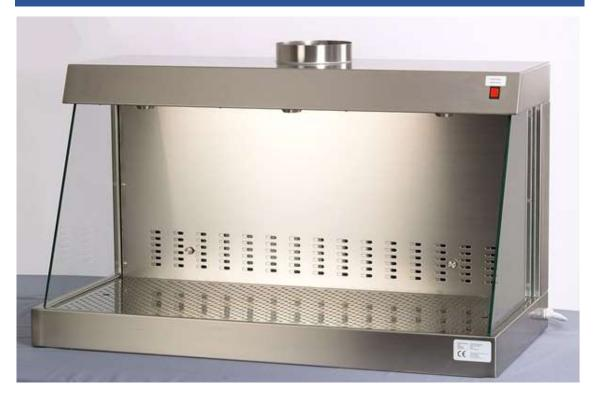
This specialized benchtop fume cupboard unit made of stainless steel (SUS304) which is to be placed on top of a table, guarantees a laboratory environment free of pollutants for example, slicing and preparing histological slide preparations. Airflow travels over the entire working area and is vacuumed out backwards, which provides optimal removal of unsanitary vapours. MAC (maximum allowable concentration) values for formalin are below target throughout the entire vacuumeffected area.
